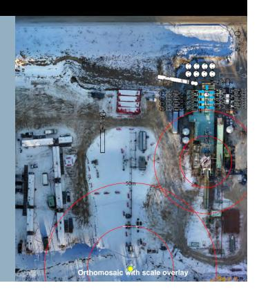
After placement of the GCPs, two grids were flown at 90m AGL with a high imagery overlap of 85% front and 70% side at a rate of 6m/sec.
