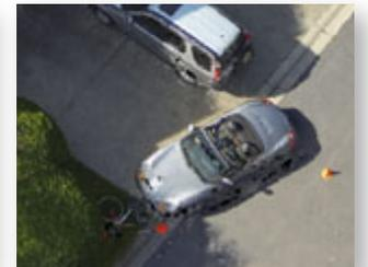
The graphics are created from 3D point cloud data comprised of millions of 3D points in space calculated from the aerial photographic data captured over the scene.
