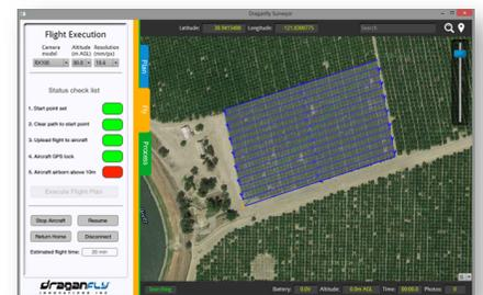
At the end of the mission, the aircraft will return home for landing by the PIC. At anytime during the mission if needed, the PIC can resume control of the aircraft or automatically return the aircraft to the designated home point.
