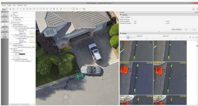
processed with Pix4D. And although the project was flown at only 12 meters, once it is processed and modeled in 3D investigators can virtually step back and view the scene from any distance, perspective, and measure the relationship of objects, skid marks etc. to less than centimeter accuracies. Keep in mind these graphic images are not photographs.
