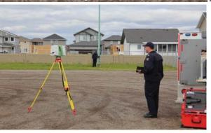
In addition to the measurements mentioned above, a terrestrial laser scanner was set up in several locations to scan over the entire scene, to be used for quality assessment of the UAV results.
