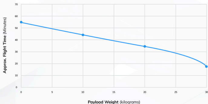
Approximate Flight Time vs Payload Weight (up to 30kg)
